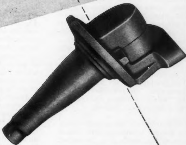
Truck Steering Knuckle Forging weighing approximately 50 pounds required special die design and forging technique to obtain required grain flow and fiber structure to resist continual shock and impact stresses.
